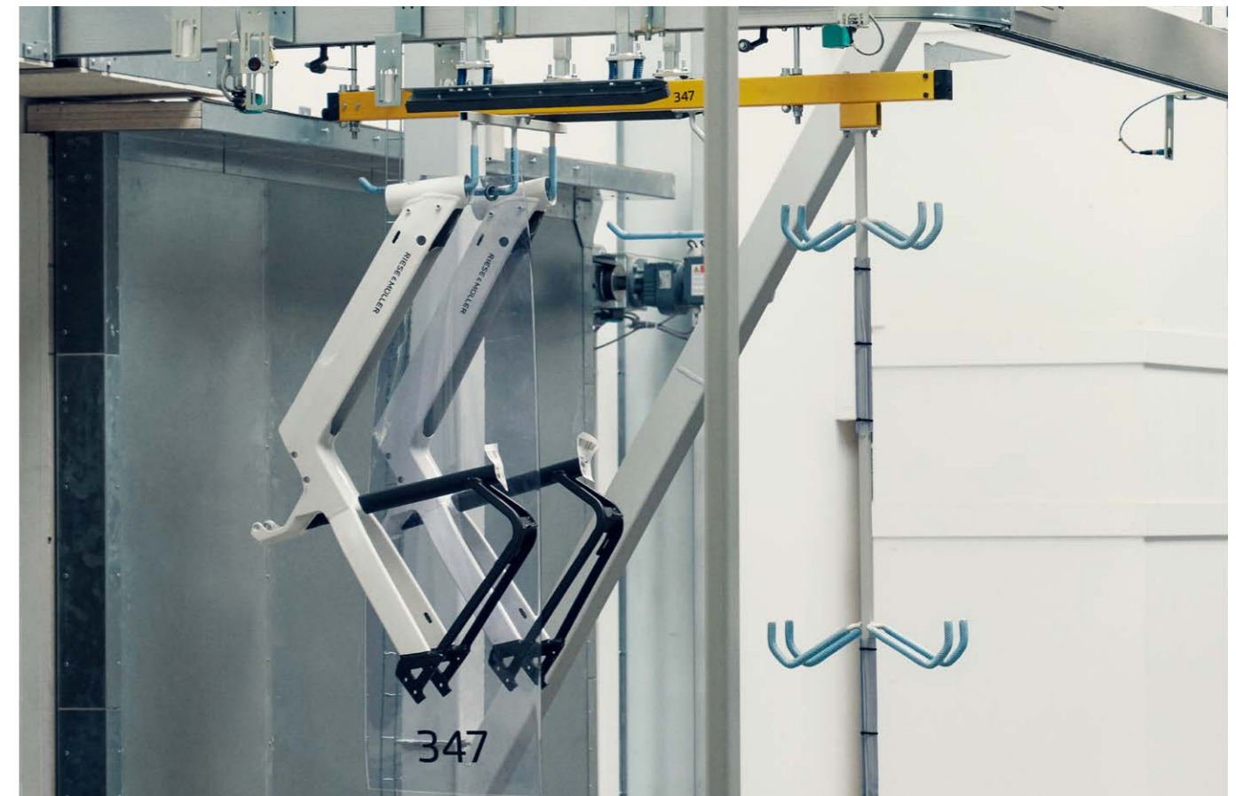
Frames are transported by the OCS transport system. Two photovoltaic plants produce almost 100% of the electricity consumed at the site.
