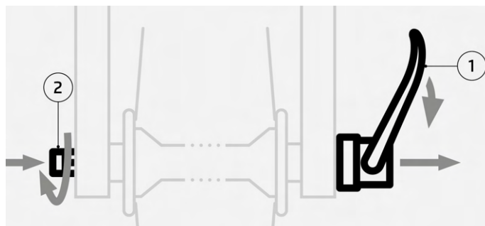
Design of the Q-Loc quick-release axle, opening
