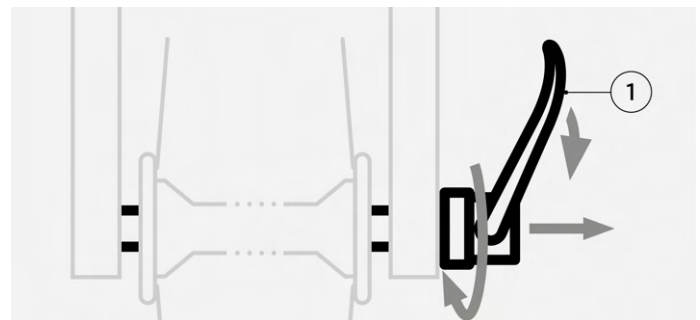
Handling the quick-release axle, opening
