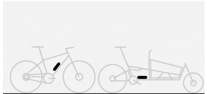
Battery on the frame
