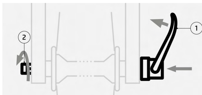
Design of the Q-Loc quick-release axle, closing
