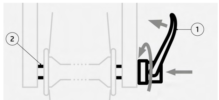
Handling the quick-release axle, closing
