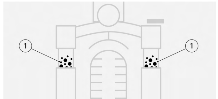
Oil leaking at the suspension fork
