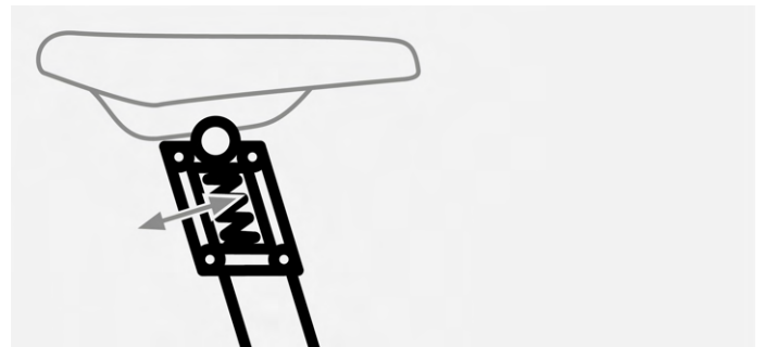
Parallelogram-shaped sprung seatpost
