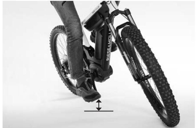
Hazardous: Crank arms not horizontal
