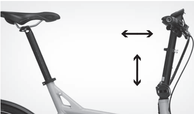
Stem with height and angle adjustment
