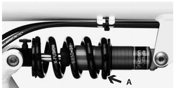
Rear shock absorber with steel spring
