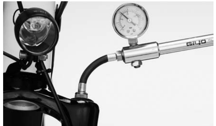
Suspension pump at the front fork
