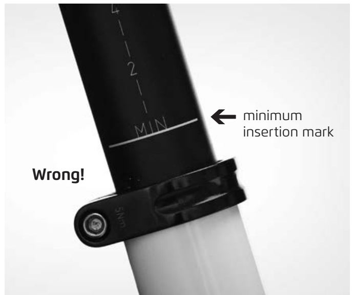
Wrong: Visible minimum insertion mark of the seat post
