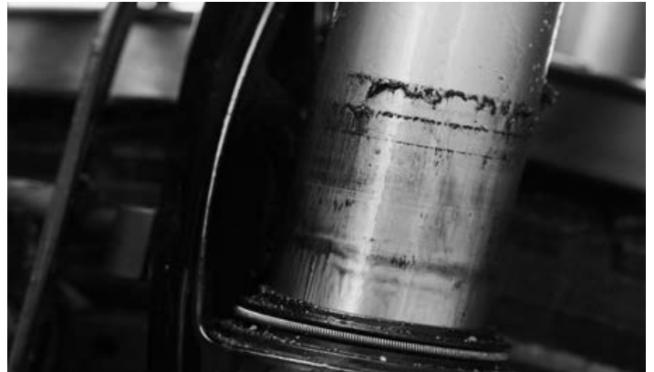
Oil leakage at the fork
